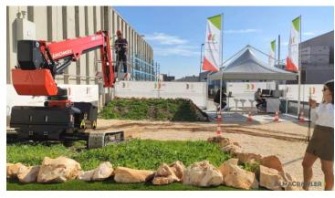
The JIBBI 1670 EVO, a 16m working height, self-propelled tracked aerial platform with telescopic boom, uses the most advanced levelling technology available on the market and represents the evolution of the JT series in terms of height, versatility of use and innovation.
